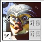
The Color Sampler tool displays color values for up to four areas.
