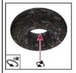
The 3D Rotate Camera tool orbits the camera in the x or y direction.
